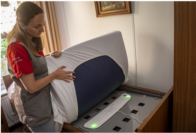
Figure 2: Momo Bedsense and its placement (source: AndersWerkenInDeZorg)
